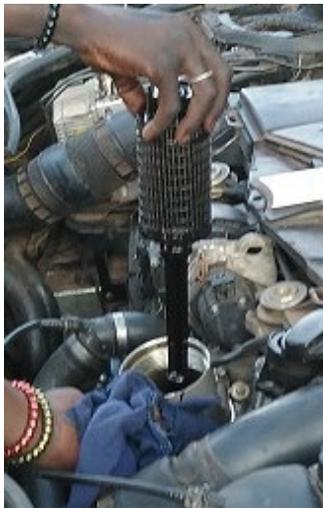
Plate 1: Removing used oil filter from engine
