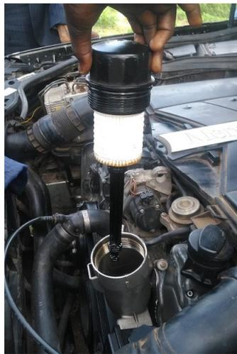
Plate 2: Changing new oil filter to engine
